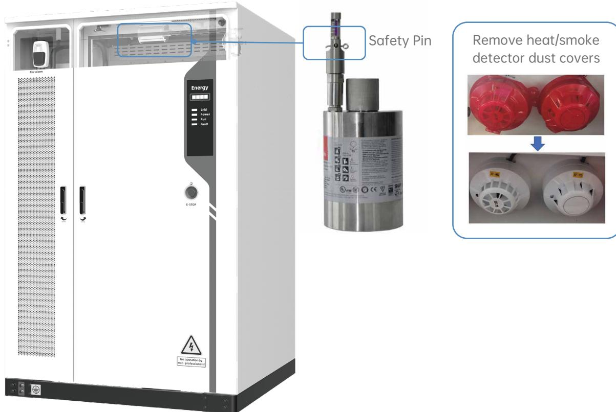
(2)Before putting the fire protection system into operation, remove all dust covers and adhesive tapes from the smoke detectors and heat detectors.
