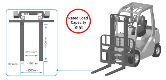
Figure 1-3 Requirements for Powered Forklifts
