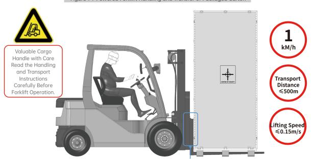
The packaging carton should be positioned tightly against the forklift fork arms.
