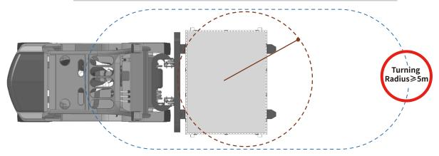
Figure 1-9 Powered Forklift Handling and Transfer of the Product
